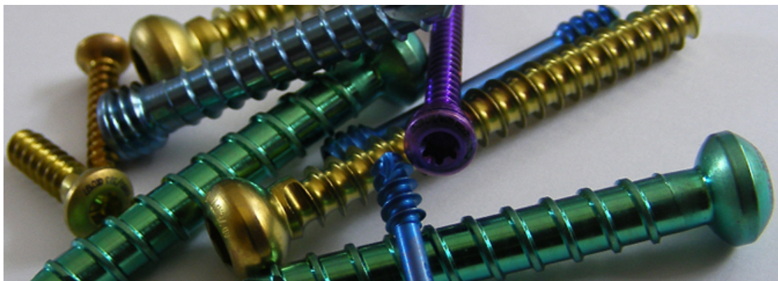
FIGURE 2.4: Colored titanium orthopedic screws. Source: Medimetal Ltd., www.medimetal.com/en
